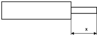
1. Measure the projection (x) of the shock absorber.
