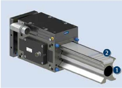
The LDx linear direct axes comprise a motor slide with integrated primary part and measuring system. The secondary part is made up of permanent magnets and is countersunk into the axis profile of the linear axis.
