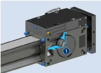
The linear module is optionally equipped with a holding brake. This holding brake is pneumatically operated. Its function is activated in a non-ventilated state. The holding brake is used to maintain the position of the linear axis in a currentless state.
